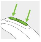
If the hearing aid is paired with a Bluetooth<sup>®</sup> enabled phone, a short press on the upper or lower part of the button will accept an incoming call and a long press will reject an incoming call – refer to chapter 12.
