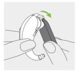
1. Place the tip of the tool in the small hole at the bottom of the hearing aid.
