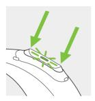
If the hearing aid is paired with a Bluetooth® enabled phone, a short press on the upper or lower part of the button will accept an incoming call and a long press will reject an incoming call – refer to chapter 12.
