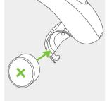
**2.** Place battery in the battery door with the flat side facing upwards.
