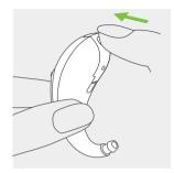
The battery is only secured when the battery door is closed correctly. Always check after closing, that the battery door cannot be opened by hand.
