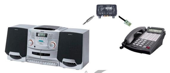
Figure 4. Sony compact disc player connected to a landline telephone via a THAT-2 telephone interface in order to allow for presentation of recorded speech materials.
